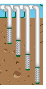
Probe can be installed at multiple depths to track the water in the full root zone.
