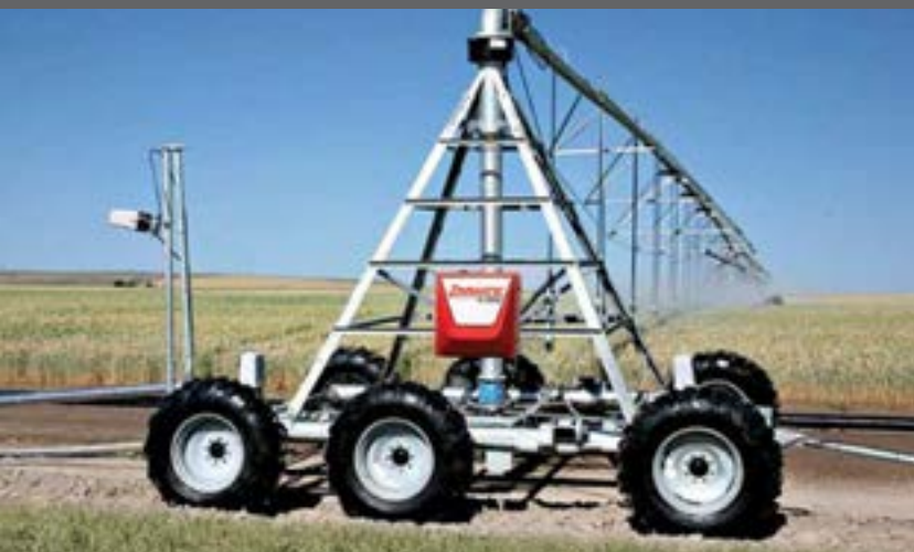
Six-wheel high traction platform
